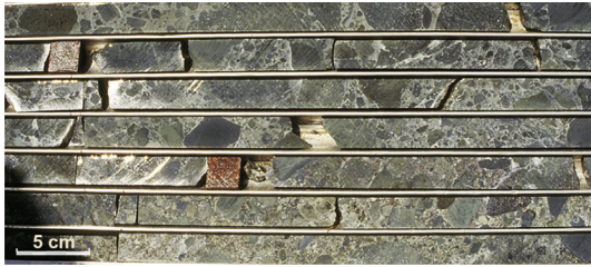
Figure 5. Volcanic breccia intersected in drill hole BD1; clasts are predominantly of basaltic rocks, while the matrix exhibits albitic alteration (after Pirajno et al., 2000).
