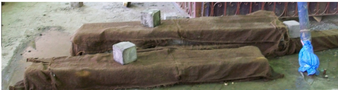
Figure 6 Curing of column specimens with wet burlap.
