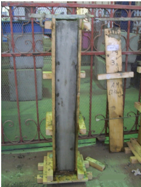
Figure 5 Demolding of column specimens.
