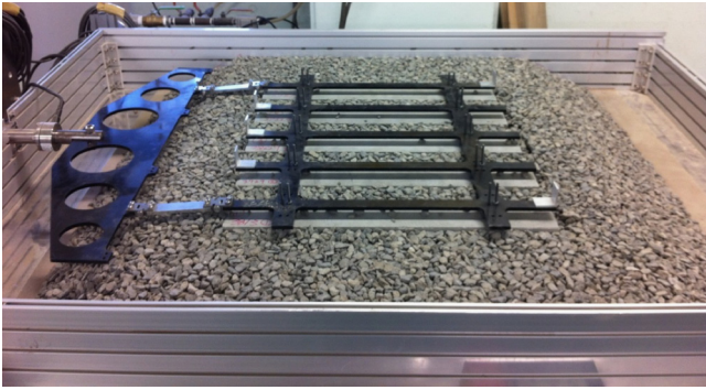
Fig. 8. Rigid frame and five rectangular parallelepiped sleepers embedded in roadbeds.
