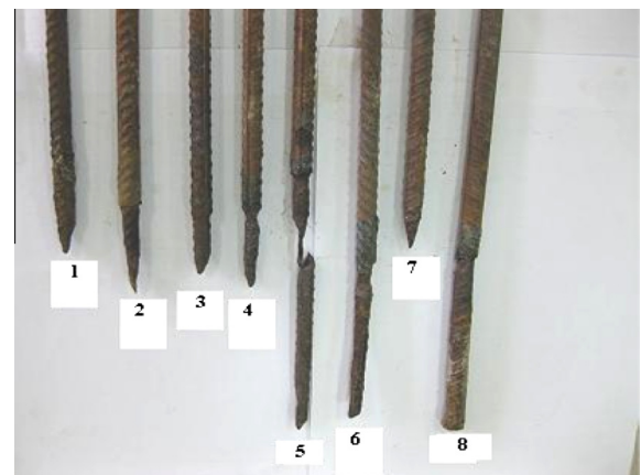
Fig. 13 Corroded steel bars due to chloride attack at the end of the test (1; COW, 2; COLW, 3;C10W, 4; C10LW, 5; C20W, 6; C20LW, 7; C30W, 8; C30LW).
