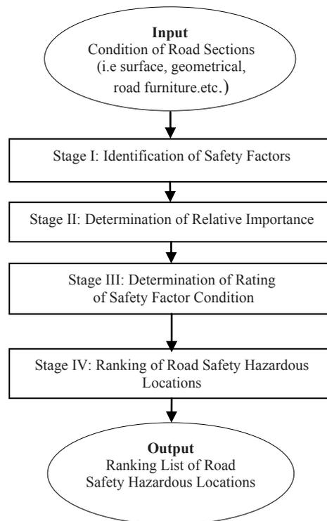
Figure 1: A Framework for Proposed Methodology for Ranking Road Safety Hazardous Locations
