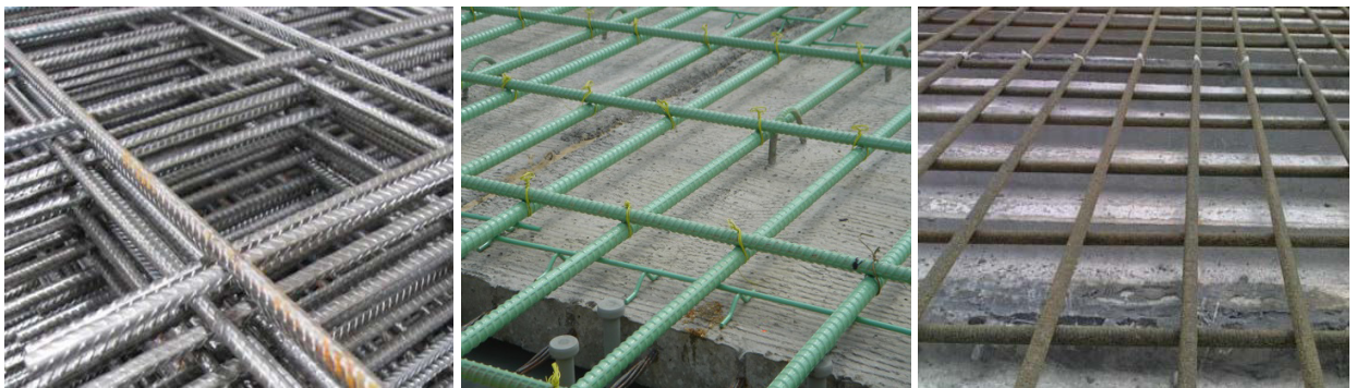
Fig. 8. Galvanized reinforcement, epoxy impregnated reinforcement and basalt reinforcement
