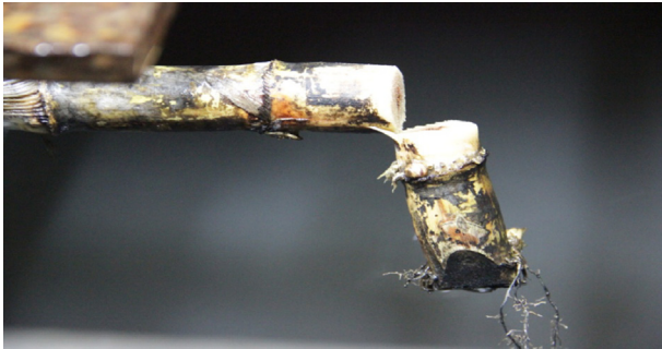
Fig. 7. Sugarcane cutting using a waterjet.
