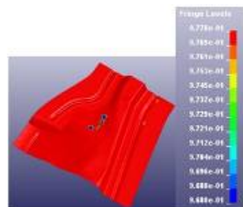
Fig. 6. The Martensite Weight Percentage at the Ending of Hot Stamping Process
