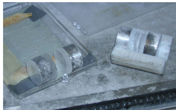
Fig. 1. Photograph showing the two aluminum inserts with the ice sample in between. Disk-shaped ice samples were grown in a freezer at CWRU using this assembly.
