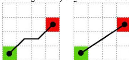
Fig. 1. Restriction of 8-connectivity searching in A\* algorithm (left) and the searching in every angle (right).
