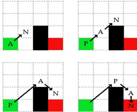
Fig. 2. Basic Theta\* algorithm. Green cell is a initial state, red cell is a goal state, black cells represent the obstacles. In the second step, the cell N has direct visibility to the cell P. That is why the cell A is ignored and the cell P and N are directly connected.
