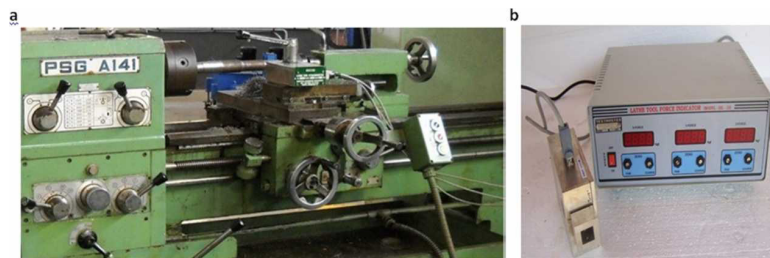
Fig. 2 (a) Experimental setup; (b) Lathe tool force indicator.
