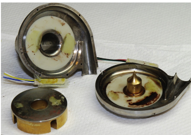
FIGURE 1. Right ventricular assist device after explantation. Fibrin and the clot can be seen inside the pump.
