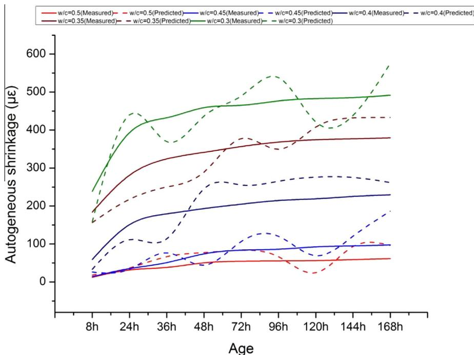
Fig. 6. Measured autogenous shrinkage values compared with predicted values.
