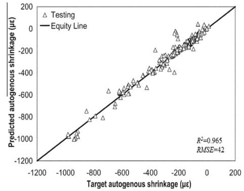
Fig. 4. Response of ANN model in predicting autogenous shrinkage of concrete for testing data [18].
