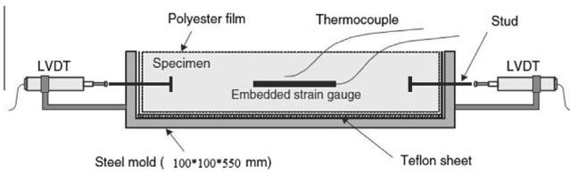
Fig. 5. Experimental set-up for autogenous shrinkage test.
