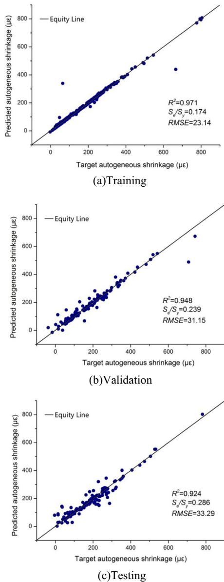
Fig. 3. Response of SVM model in predicting autogenous shrinkage of concrete: (a) training; (b) validating; and (c) testing.
