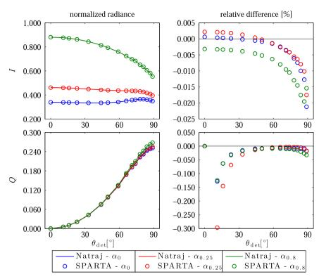
**Fig. 9.** Comparison between SPARTA and the tabulated values by Natraj et al. [46] for Case 4, for  $\tau = 0.5$ ,  $\mu_0 = 1$ , and  $\phi = 0^\circ$ . Left: normalized Stokes vector at the TOA (line – Natraj, circles – SPARTA). Right: Relative differences in percent of SPARTA as correlated to the benchmark results.
