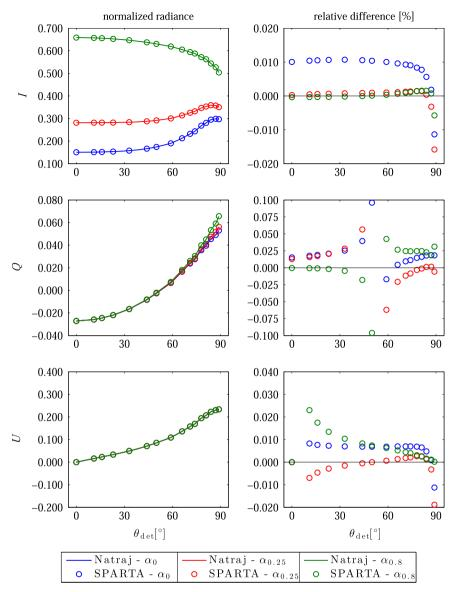
**Fig. 7.** Comparison between SPARTA and the tabulated values by Natraj et al. [46] for Case 3, for  $\tau = 0.5$ ,  $\mu_0 = 0.8$ , and  $\phi = 90^{\circ}$ . Left: normalized Stokes vector at the TOA (line – Natraj, circles – SPARTA). Right: relative differences in percent of SPARTA as correlated to the benchmark results.
