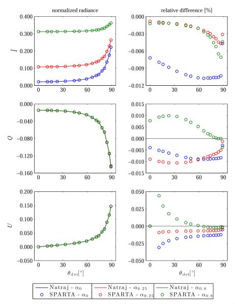
**Fig. 5.** Comparison between SPARTA and the tabulated values by Natraj et al. [46] for Case 2, for  $\tau = 0.1$ ,  $\mu_0 = 0.8$ , and  $\phi = 90^{\circ}$ . Left: normalized Stokes vector at the TOA (line – Natraj, circles – SPARTA). Right: relative differences in percent of SPARTA as correlated to the benchmark results.
