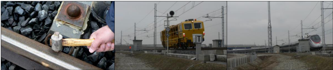
Fig. 3. Type of excitation: impact hammer, maintenance vehicle and high speed train
