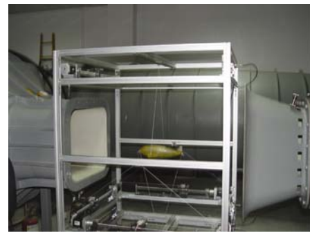
Fig.5 WDPSS-8 suspension system in wind tunnel.
