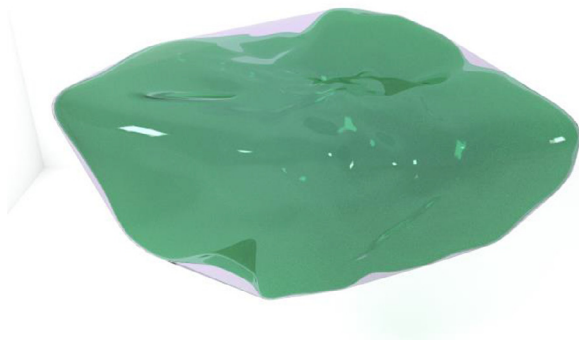
Fig. 14. 3D SH reconstruction of a coarse aggregate particle formed from blast furnace slag. The particle, rendered in green, is reconstructed by SH expansion to degree 16. The particle’s convex hull is rendered in purple, and is used to compute the particle’s convexity.
