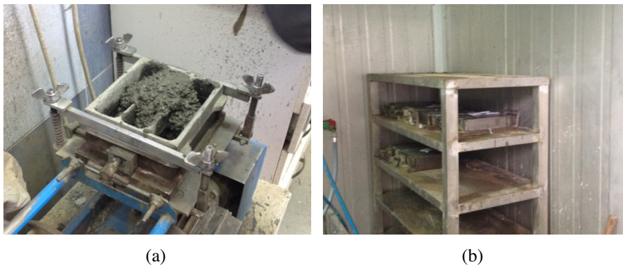
Fig. 1 (a): Casting concrete into specimen prism, (b): The specimen at moist air room.
