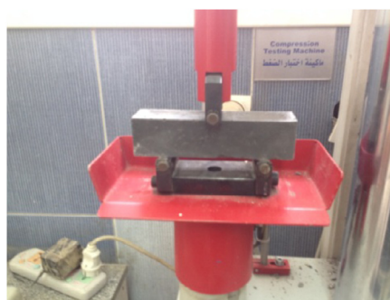
Fig. 3 Arrangement of loading for determination of flexural strength.
