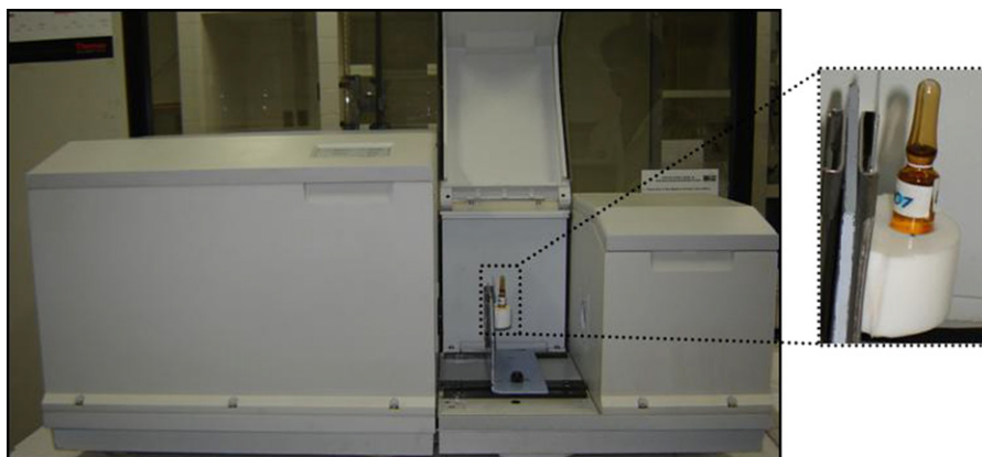
Fig. 1. NIR spectrophotometer with the lab-made teflon holder which was used to support the ampoules in the spectrophotometer sample compartment.
