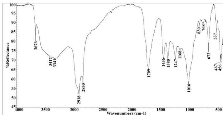
Fig. 6. FTIR spectrum in DRIFT modality of sample 4 (powder scraped from the rubberized fabric).
