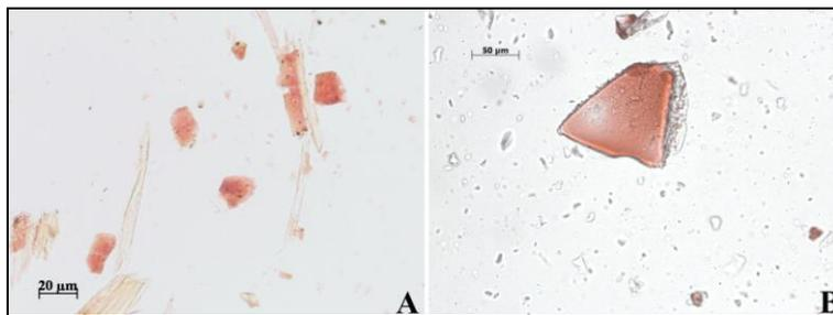
Fig. 2. Microphotographs in transmitted light of the sample nr. 2 (A) and of Brazil wood lake (B) prepared in our laboratory from Brazil wood.
