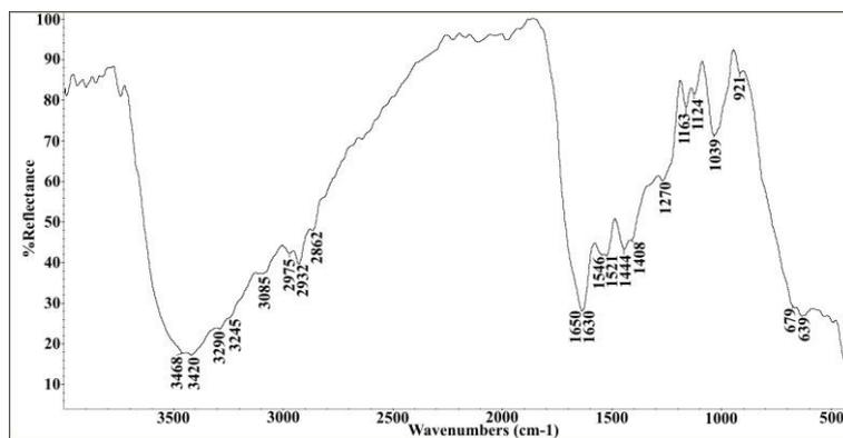
Fig. 7. FTIR spectrum in DRIFT modality of sample 2.
