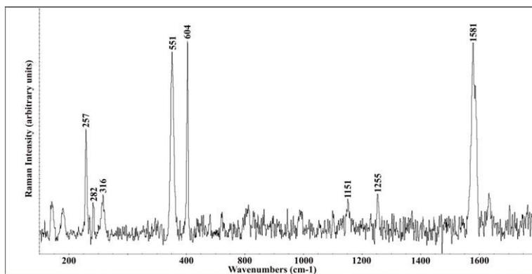
Fig. 3. Raman spectrum of indigo, found in the blue samples.
