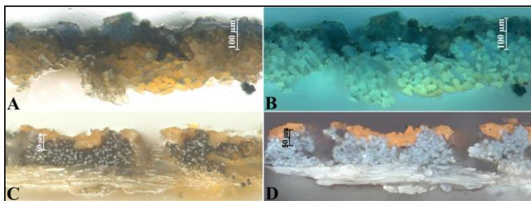
Fig. 5. Microphotographs of samples 8 (A, B) and 7 (C, D), under reflected light (A, C) and UV fluorescence (B, D).
