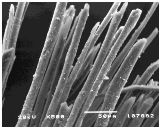
Fig. 9. SEM image of silk fibers
