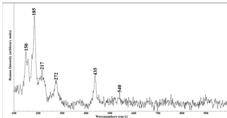
Fig. 4. Raman spectrum of malachite, found in the green samples from the trees and from the hills.
