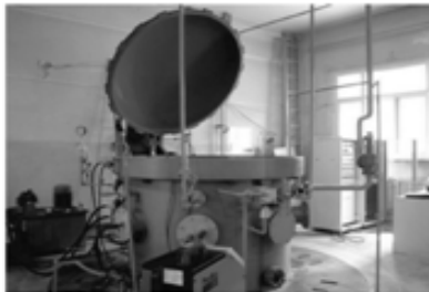
Fig.2 Underwater welding test device
