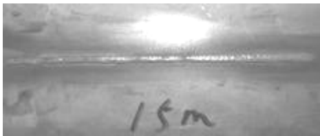
(c) back side of butt weld
