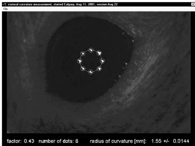
Fig. 1. Screen dump of the C++ program that located the first Purkinje images created by a circular arrangement of eight infrared LEDs on the corneal surface in a highly magnified video image of the mouse eye in vivo. The radius of curvature was automatically determined by the program, based on a prior calibration with ball bearings of known radius. Ten measurements acquired in 0.4 s had a standard deviation of the radii of curvature of about 15 \mu\text{m} .
