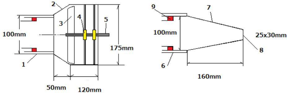
Fig.3. Design of turbine (a) and nozzle(b): 1. Outer casing of combustor, 2 Shroud of turbine, 3. Turbine blade, 4. bearing, 5 10mmdiameter steel shaft, 6. Outer casing of combustor, 7. converging duct wall, 8. 20mmx30mm square jet, 9. Gypsum shield(removed)
