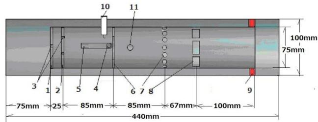
Fig.2. Design of Combustor: 1. Front room, 2. wall of front and pilot room, 3 a hole 4. pilot fuel line, 5. Pilot fuel outlet, 6, choke, 7. Holes of primary combustion, 8. Square holes for the second combustion and cooling, 9. Shield of gypsum, 10. Spark plug, 11. main fuel line
