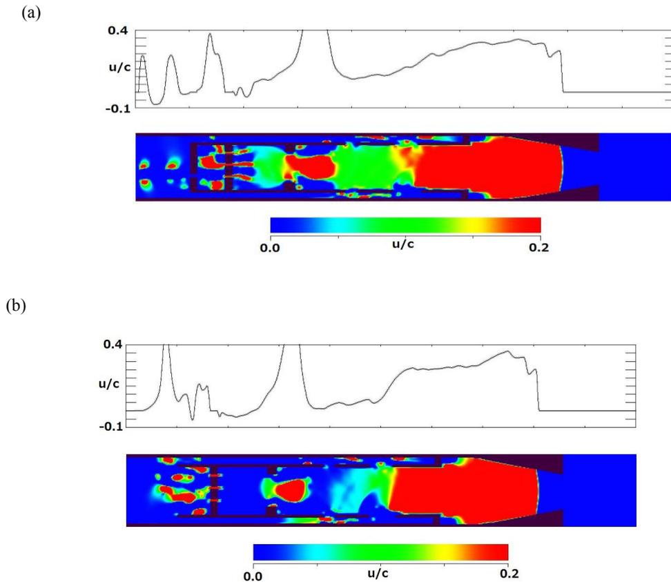
Fig.4.Shock wave analysis (a) velocity distribution with front chamber, (b)velocity distribution without front chamber where no flows in the front chamber
