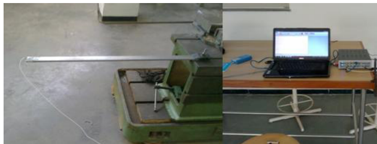
Fig. 5 Experimental set up for crack detection of a cantilever beam with single crack
