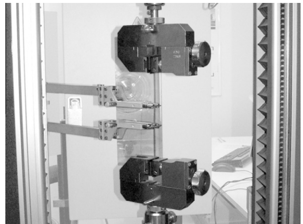
Fig. 2. Experimental setup used for tensile tests.
