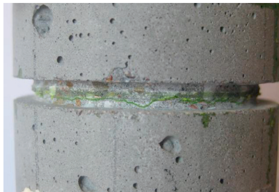
Figure 14. Crack formation of concrete cylinder in the notch.
