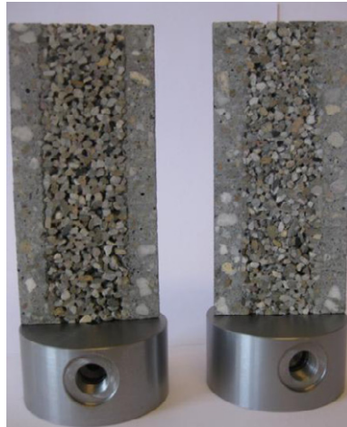
Figure 9. Bone-like concrete; a new hierarchical material is made in which sponge-like core is surrounded by solid concrete.
