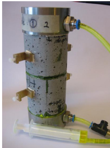
Figure 12. SHA was manually injected into porous layer at the top side.
