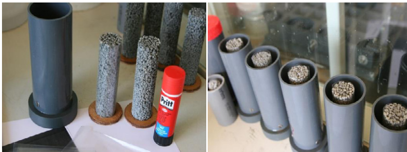
Figure 8. Casting preparation where porous concrete cylinder was placed in the center of the mould and normal strength self compacting concrete was poured around.
