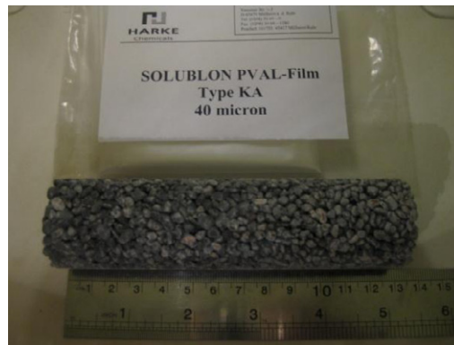
Figure 7. Porous concrete cylinder that would be used as porous core in PNC samples.
