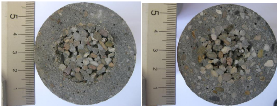
Figure 9. Bone-like concrete; a new hierarchical material is made in which sponge-like core is surrounded by solid concrete.
