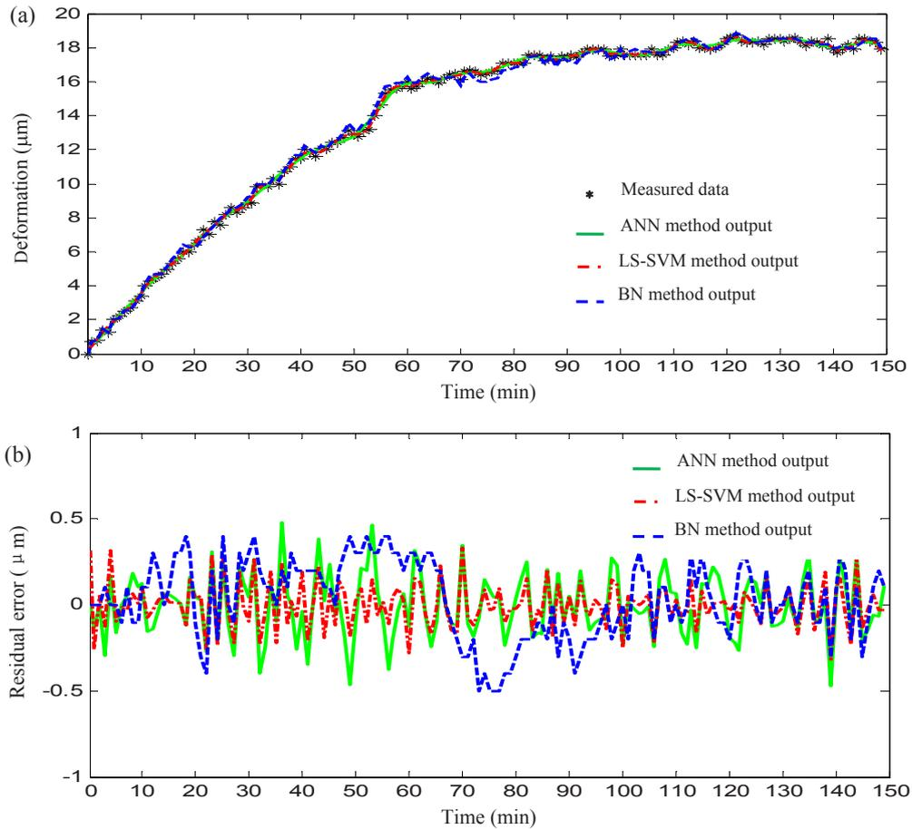
Fig.4. Modeling comparison results in radial direction. (a) Deformation; (b) Residual error
