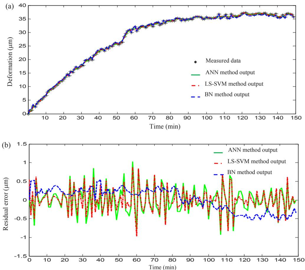
Fig.3. Modeling comparison results in axial direction. (a) Deformation; (b) Residual error
