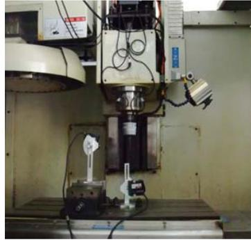
Fig.2. Synthetic error measurement
