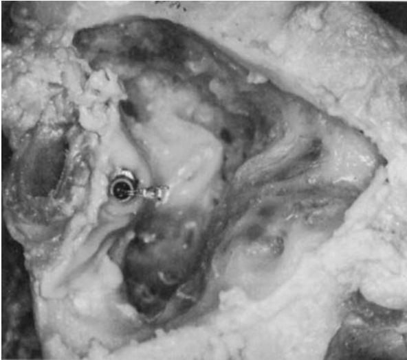
Figure 11. Sensor implanted in a fresh temporal bone. This situation was used for determination of acoustic free-field frequency response in Figure 12.
