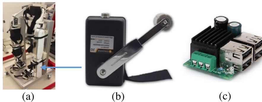
Figure 2 (a) Exo-Leg and actuator position (Gastriland, n.d.), (b) HCG (Aliexpress, n.d.), (c) DC–DC converter (Suntekstore, n.d.).
