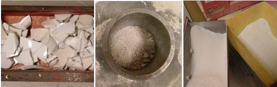
Fig. 1. Raw ceramic waste was first broken with a hammer into 50–150 mm fragments, then crushed down to 30 mm particles, and finally ground.
