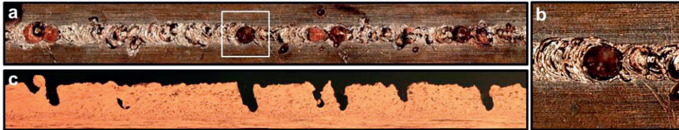
Fig. 1. Welded copper sample, Cu-ETP, v = 6 m/min, P = 1500 W, d_f = 100 \mu\text{m} . (a) Weld seam surface with melt ejections; (b) Enlarged image of a melt ejection; (c) Corresponding longitudinal cross section.
