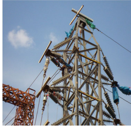
Fig. 5. Calibrated load cells attached to the composite cross arm
