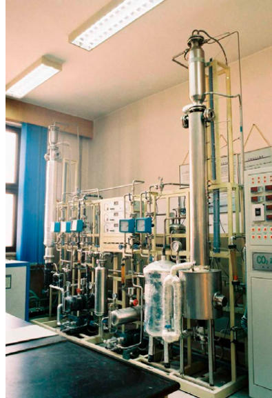
Fig.3 Pilot plant facility for CO 2 absorption in Tsinghua University.
