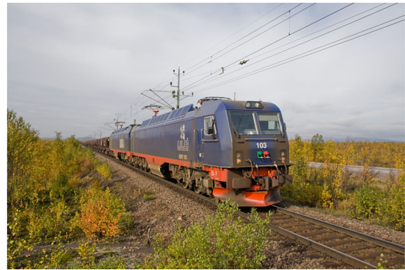
Fig. 3. IORE locomotive used for real friction coefficient measurements.
