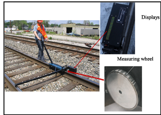
Fig. 5. The tribometer utilised for the friction coefficient measurements.
