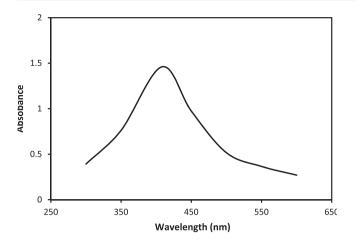
Figure 3 UV–Vis spectrum of Ag nanoparticle colloid in 1:4 ratio of  $AgNO_3$  to  $NaBH_4$ .
