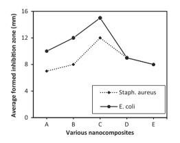
Figure 8 Scatter plot of inhibition zone *versus* various PVA/ PANI/Ag nanocomposites at different concentrations of Ag nanoparticles: 5% (A); 10% (B); 15% (C); 20% (D); 25% (E).
