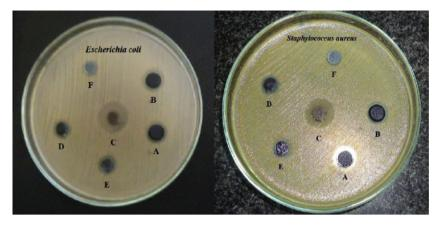
Figure 7 Antibacterial activity of various nanocomposites against two pathogenic strains; *E. coli* and *Staph. aureus* shown by the paper disk diffusion method; 5% (A); 10% (B); 15% (C); 20% (D); 25% (E).
