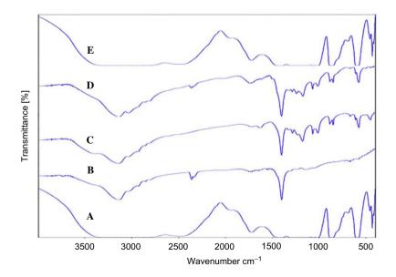
**Figure 4** FT-IR spectra of prepared nanocomposites at different concentrations of silver nanoparticles; 5% (A); 10% (B); 15% (C); 20% (D); 25% (E).
