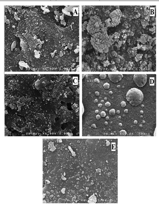
Figure 6 FESEM images of prepared nanocomposites at different concentrations of silver nanoparticles; 5% (A); 10% (B); 15% (C); 20% (D); 25% (E).
