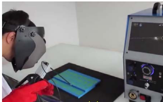
Fig. 1. AR system for welding. Source: http://soldamatic.com.br/asoldamatic.html
