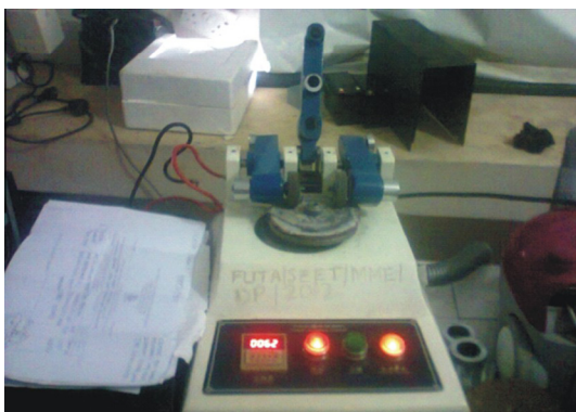
Fig. 1. Taber abrasion machine utilized for wear testing of the composites produced.
