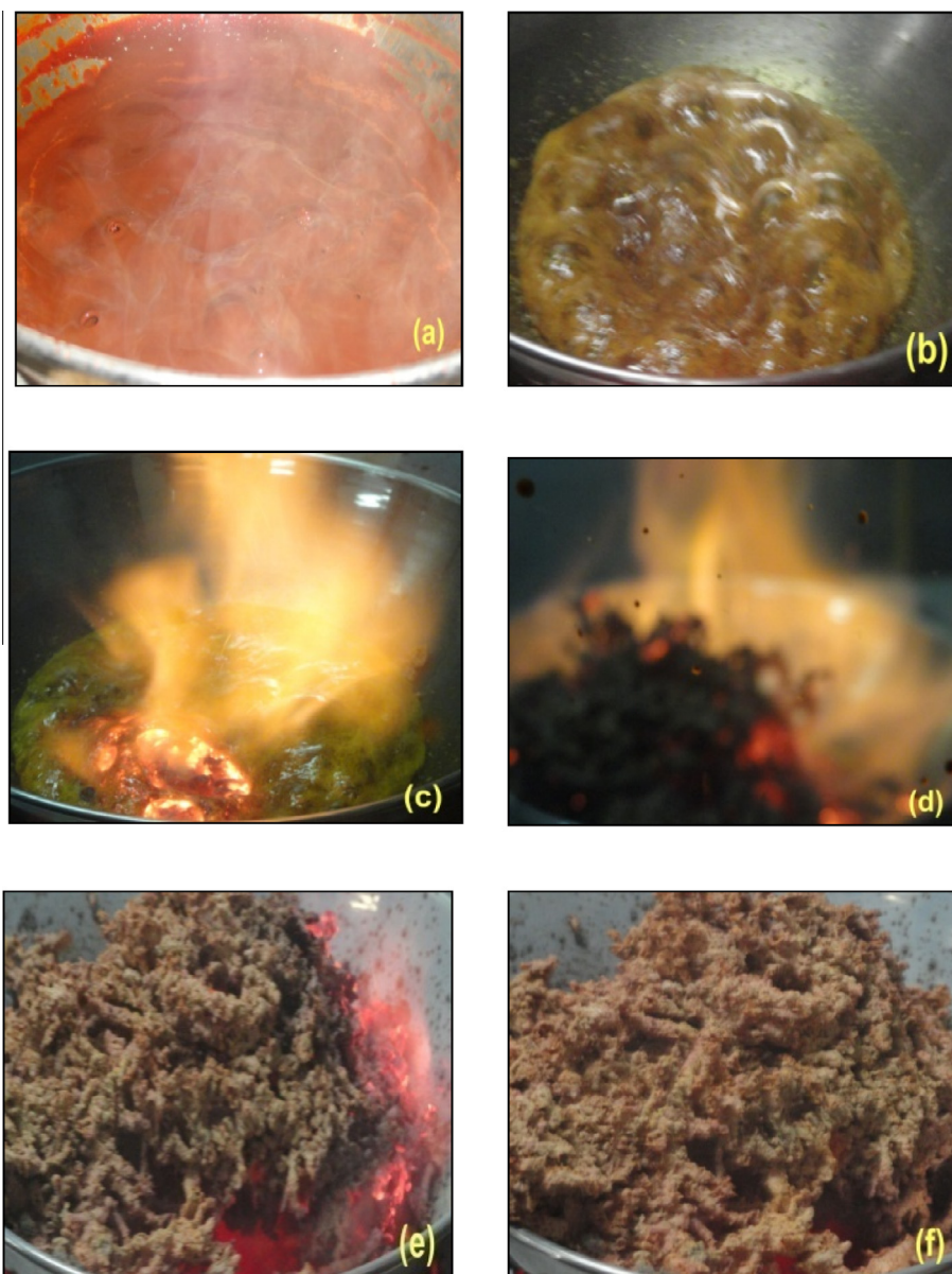
Figure 1 Sol-gel auto-combustion process for preparation of soft magnetic material ( \text{MgFe}_2\text{O}_4 ): (a) sticky sol, (b) condense gel heated at 120\text{ }^\circ\text{C} , (c) auto combustion started, (d) full combustion at 250\text{ }^\circ\text{C} , (e) slow down combustion, and (f) foaming powder material of \text{MgFe}_2\text{O}_4 .
