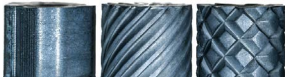
Fig. 2. PCD Milling tools: (left) Geometry A; (middle) Geometry B; (right) Geometry C.
