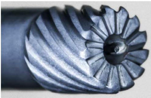
Fig. 5. PCD torus milling tool (diameter 1.8mm) with optimized geometry.
