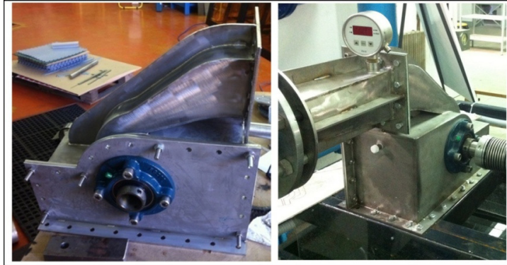
Fig. 3. Two different views of the Cross-Flow turbine prototype.
