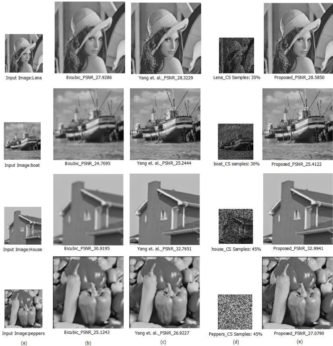
Fig.4. Visual comparison of the results; Column (a) Low resolution downsampled input image; (b) Results of Bicubic method; (c) Results of Yang et al.'s method; (d) Compressive samples given as input to the proposed method; (e) Results of the proposed method.
