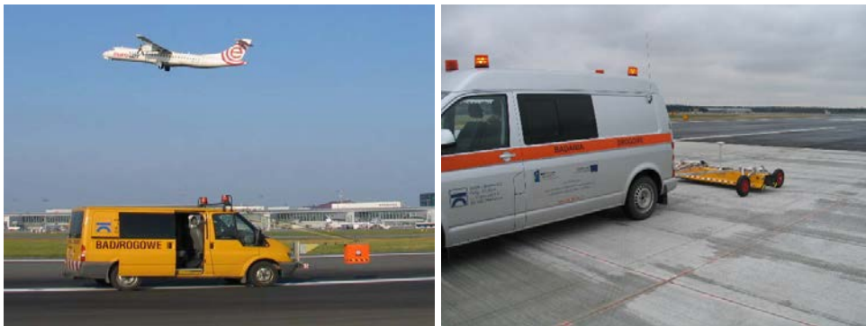
Fig. 1. The GSSI system with a high-frequency 2.2 GHz antenna (right); 3D system from Radar AS.
