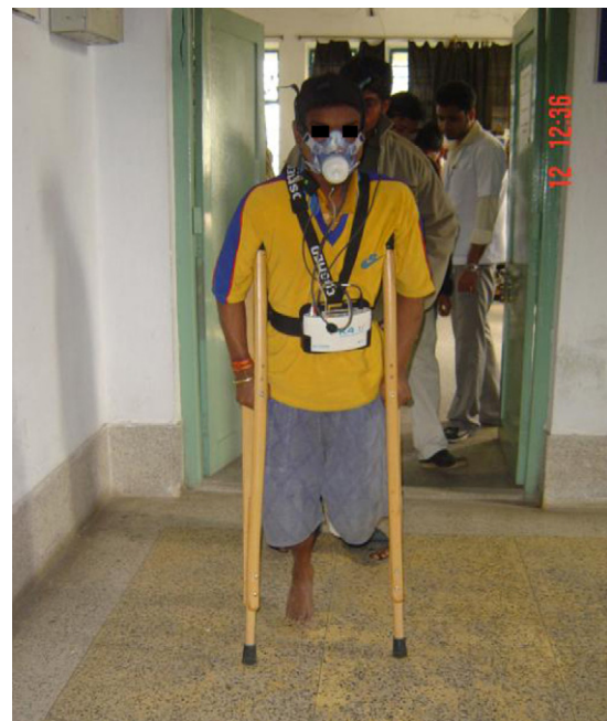
Fig. 2. The K4b2 system fitted and the subjects performed the test with Crutches without Prosthesis.
