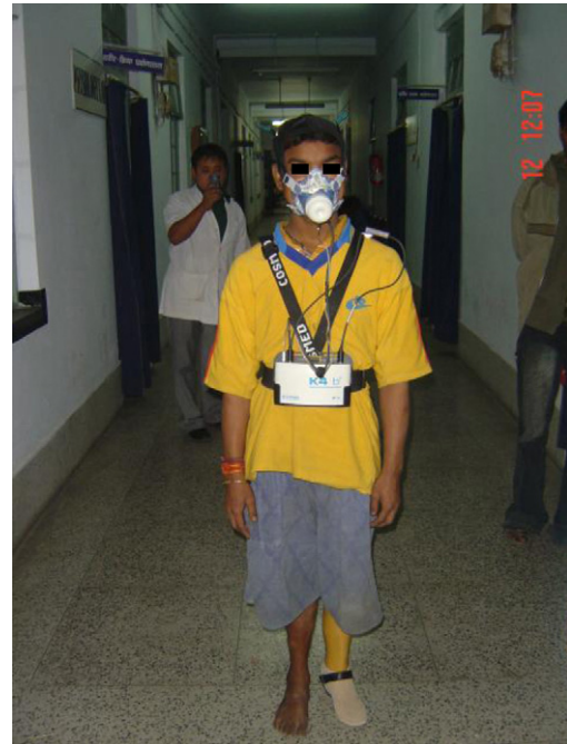
Fig. 1. The K4b2 system fitted and the subjects performed the test with Prosthesis.
