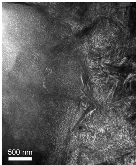
Fig. 20. TEM micrograph of Ip C-S-H (left) and Op C-S-H (right) in the alkali-activated wPc-30% pfa paste reacted for 4 years. The Op C-S-H has the foil-like morphology that is characteristic of C-S-H(I). The Ip C-S-H has the fine-scale morphology that is typical of alite Ip C-S-H.
