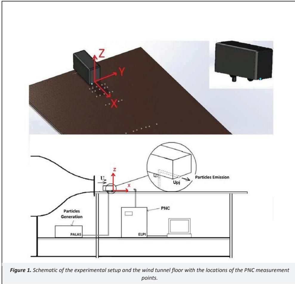
Figure 1. Schematic of the experimental setup and the wind tunnel floor with the locations of the PNC measurement points.
