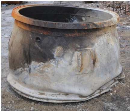
Fig. 3. Lower part of the reactor.
