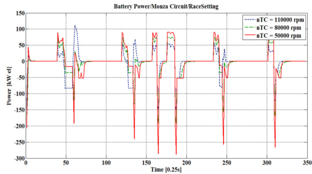
Fig. 5. Battery power, history with time for different fall speeds of the turbocharger in race setting.
