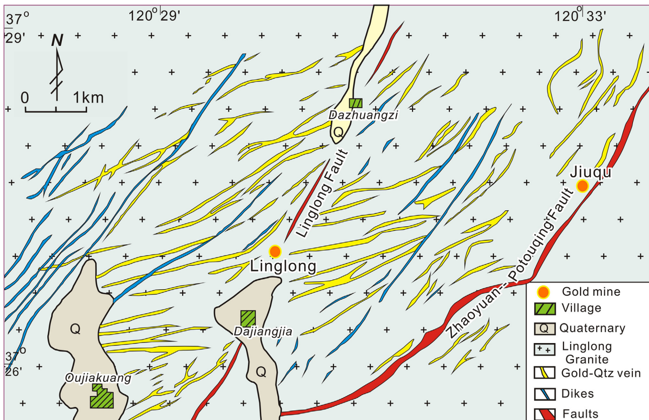
Figure 4. Detail structural map of the Linglong goldfield after Zhuang and Wang (2009) showing the extensive vein system presently being mined by a number of underground operations. The major ore controlling structure in the goldfield is the NE-striking Zhaoyuan-Potouqing ductile-brittle reverse shear zone, with NE-trending gold-bearing extensional veins being continuous along strike for as much as 5 km within a series of en-echelon brittle faults. The NNE-striking Linglong normal fault is a late- to post-gold feature that cuts through the goldfield.
