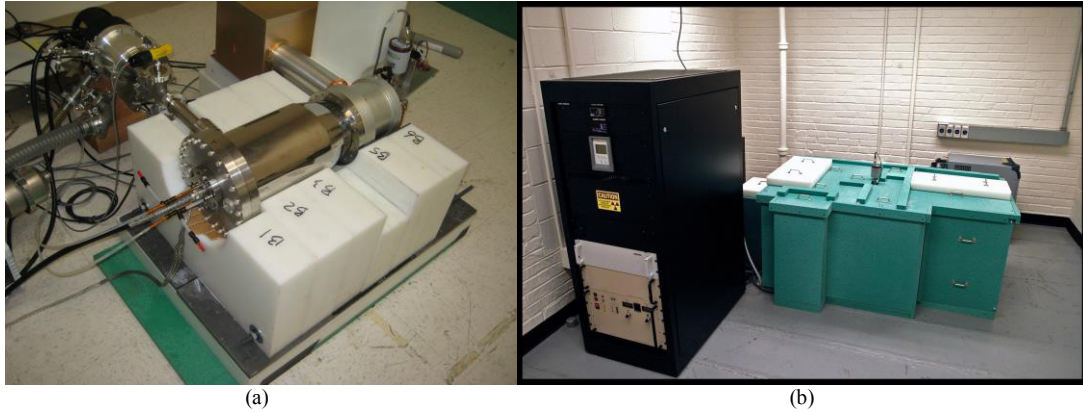
Fig. 4. (a) Moderated DD-109. Moderation of fast neutrons is accomplished by using high density polyethylene. Top of HDPE moderator shell has been removed. (b) Shielding of thermal neutrons is accomplished by borated polyethylene surrounding the HDPE.
