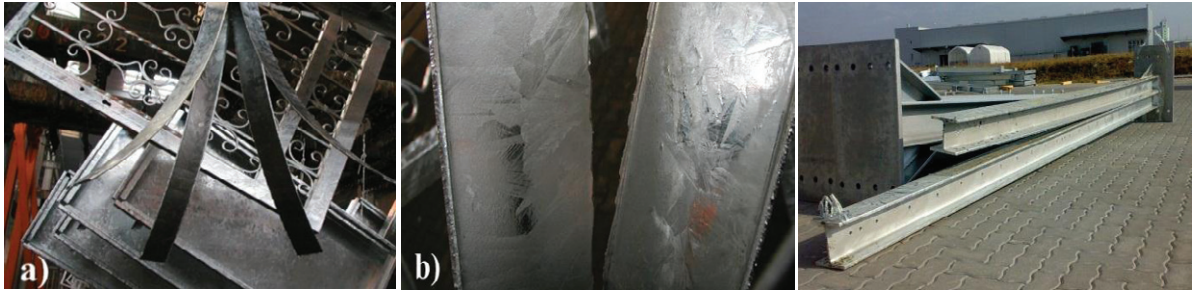
Fig. 3. Steel becoming brittle due to bending – (a) view, (b) detail
